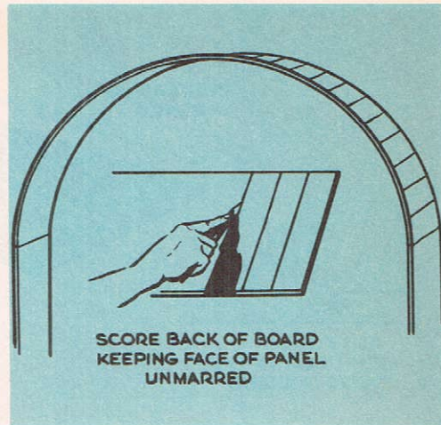
Fig. 14. Plasterboard can be bent to form rounded corners by scoring the back of the board with a knife.
