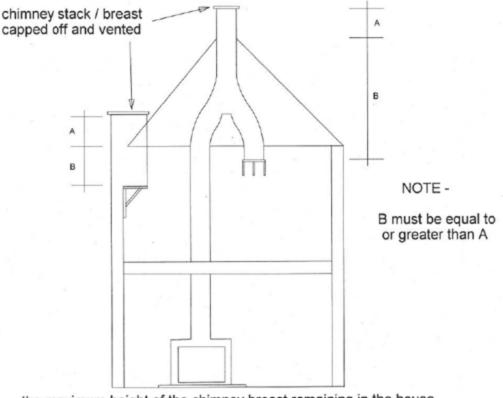
the maximum height of the chimney breast remaining in the house (below the roofline) must be equal to or greater than the hight of the brickwork in the stack above the roof
