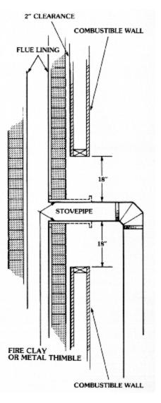
about 2 inches with the crimped (male) end pointing down into the next piece. This arrangement will prevent creosote leaks. When connecting a stove to a chimney, it is preferred to have only one 90 degree elbow. Two can be used, however, when necessary.
