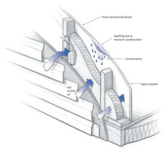
When the vapor retarder is on the interior wall in hot, humid climates, warm, moist air that enters the wall cavity can accumulate on the cold interior wall board, which swells and disintegrates.
