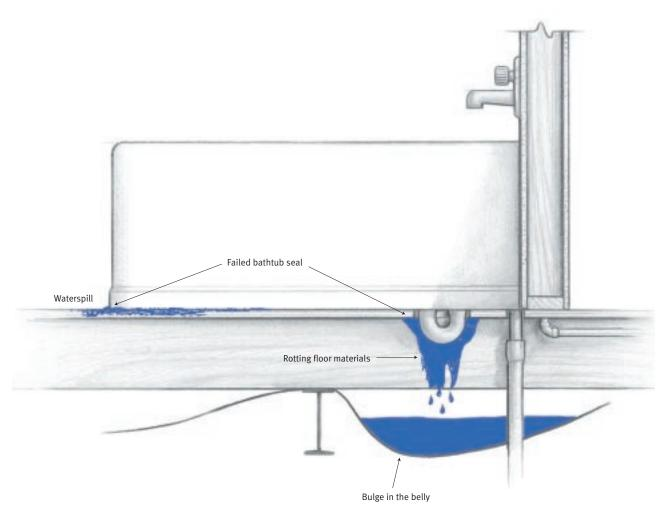
When seals around tubs fail, water drains into the floor cavity and pools on the bottom board. Unchecked, the leaks can rot out floor materials.
