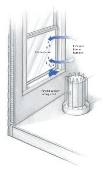
In winter, excessive interior humidity causes water to condense and run down inside the surface of the window glass and damage the sill. Unvented combustion space heaters that give off a good deal of moisture are sometimes the culprit.
