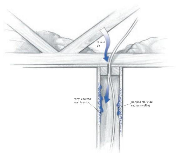
Humid outside air can enter an interior wall cavity through poorly sealed holes for wiring. Moisture condenses on the cold wall. The moisture cannot dry through the vinyl, causing the interior wall to swell.
