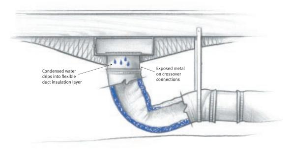
Exposed metal on crossover connections condenses water that can seep into the flexible duct insulation layer. The water builds up until its weight kinks the flexible duct, restricting airflow.
