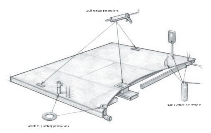
The floor is a natural moisture and air barrier. Keep it intact by sealing all floor penetrations with the appropriate sealant or gasket.
