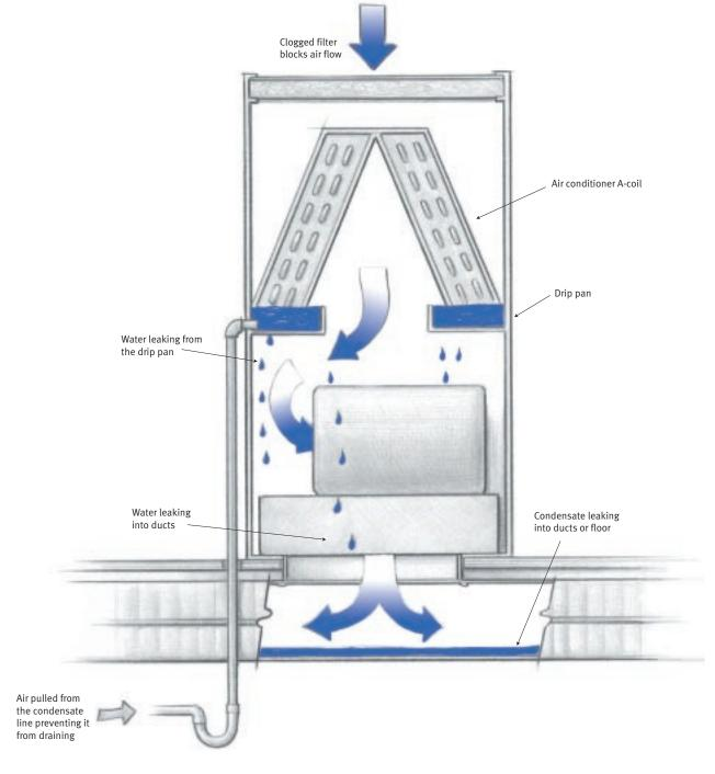
A clogged air conditioner filter blocks return airflow, and the "starved" air handler fan sucks water out of the drain line. Water spills into the air handler cabinet, leaking into ducts and seeping into the floor.
