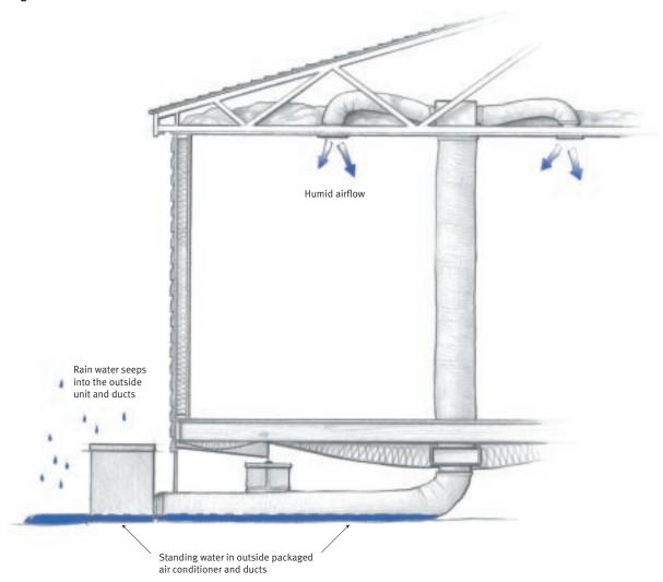
Heavy rains may drive water into the outside air conditioner's main supply and return ducts. When the air conditioner runs, moist air and often moldy odors are the result.
