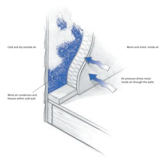
Static and vapor pressure drives moist inside air through the walls, where it condenses on the insulation and freezes. The frozen walls are cold to the touch, and the home will not feel warm.
