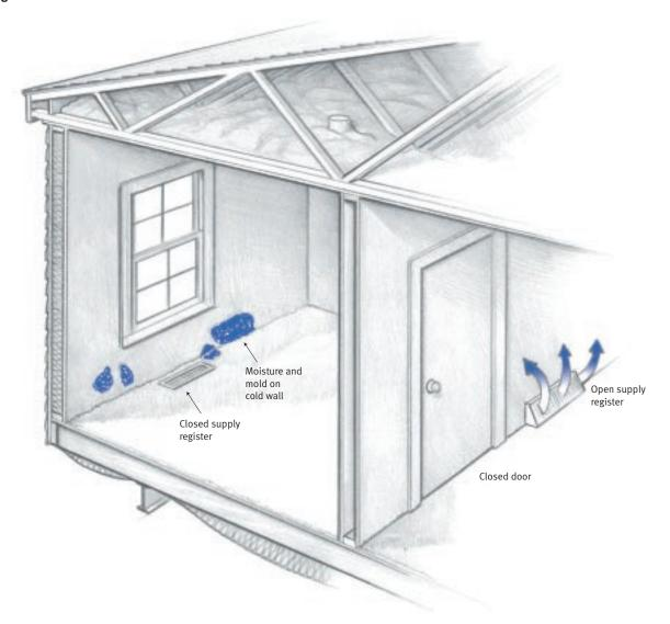
When the supply grilles are closed, warm air cannot enter a closed-off room. The inside air will become cold enough to significantly raise the relative humidity level in the room, supporting mold growth.
