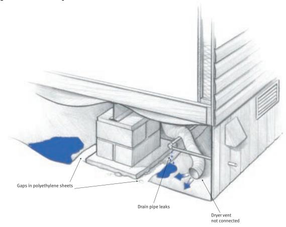
Figure 3.13 Crawlspace Moisture Control and Ventilation
