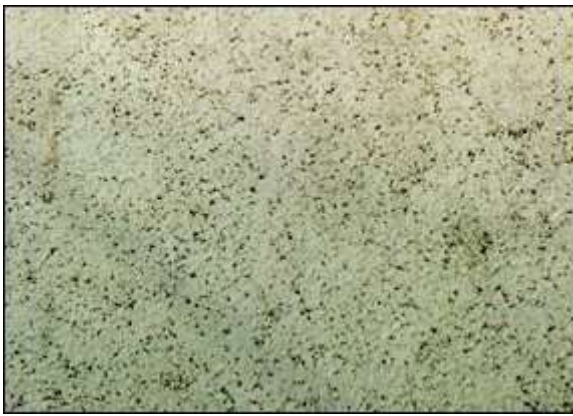
Figure 4. Closeup of sooty mold colonies on surface of propane tank.
