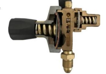
The internal workings contain springs and a rubber diaphragm, over time the components may deteriorate resulting in less effective pressure control.
