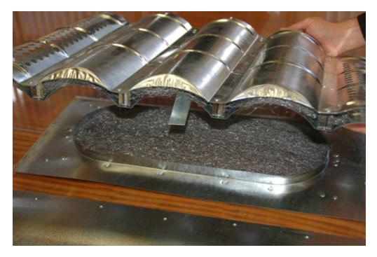
Vents accepted by the OSFM have provided testing information that was conducted by an accredited fire testing laboratory. Testing has evaluated the ability of a vent to resist intrusion of embers and flames. Since vents can be exposed to embers, without being exposed to flames, separate tests are run.
