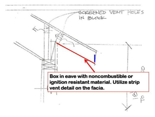
An example of soffit /eave strip vent in the fascia board. This design is on a home, and so was probably approved for use by the local building official.
