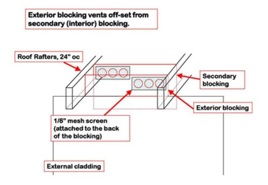
In this diagram, interior and exterior blocking with an alternative design for off-set friezeblock vents. The interior surfaces could be coated with intumescent paint.
