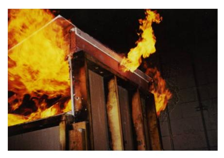
Example of fine fuels in attics. Embers will ignite finer combustible materials which, if sustained, can in turn ignite larger structural wood members and other combustibles in these spaces
